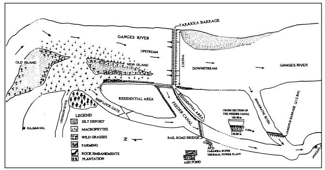
Figure 2. Detailed sketch map of the Farraka Barrage Complex.
