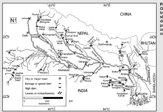
Figure 3. Map of the Ganges river system in India and Nepal showing barrage, high dam, and embankment projects (planned, underway, and already constructed).
